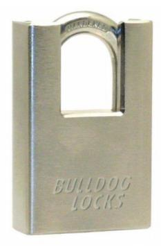
Solid steel body and shackle, case hardened and chrome plated Raised shoulders for added shackle protection Double ball bearing locking mechanism Key removable only when shackle is locked 5 pin tumbler mechanism 2 keys per lock Available keyed to differ (KD) or keyed alike (KA) Individually boxed Key blank TM2 for models 934 and 935 Key blank TM1 for model 936
